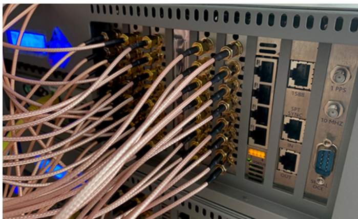
C50 HRC Physical Port Placement and Assignment Example: 20 Radio Ports and 4 10Gbps Ethernet Ports
