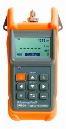
\*\*OPM-50 paired with SLS-50 Intelligent Stabilized Laser Source can be used to identify fibre, measure attenuation and loss, verify continuity and evaluate fibre link transmission quality.\*\*
