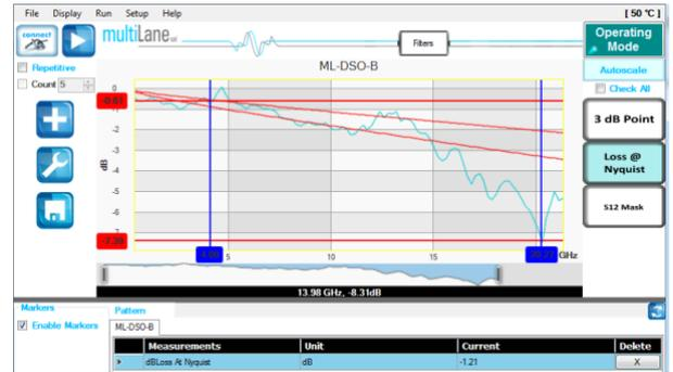
Figure 2: Adaptive channel equalization for up to 14dB loss at Nyquist
