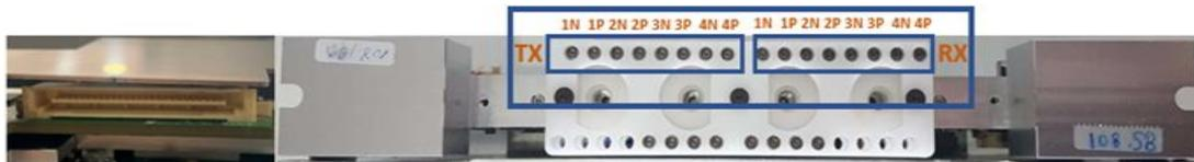
Figure 5: AT4039D Pinout. closest to the backplane connector is TX1N
