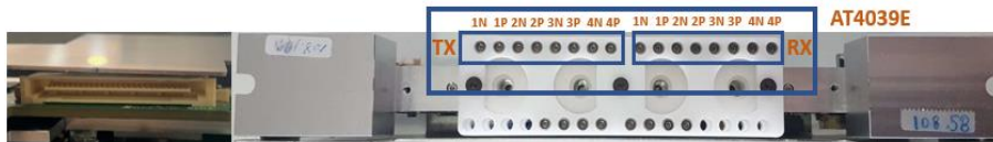
Figure 4: AT4039E Pinout. Closest to the backplane connector is TX1N
