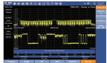
**Figure 6:** LTE Power vs Time chart provides both time-domain and spectrum analysis.
