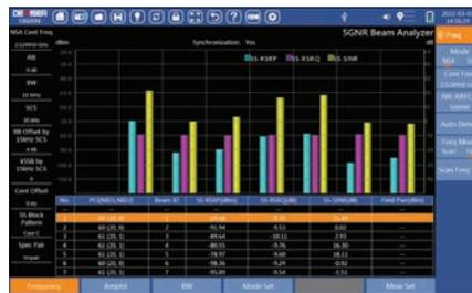
**Figure 5:** 5G NR beam analysis measures up to 8 beams at once.
