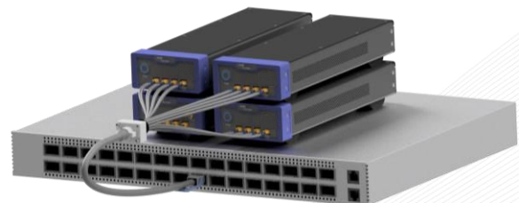
Figure 3 Switch Testing using 4 Pulsars.
