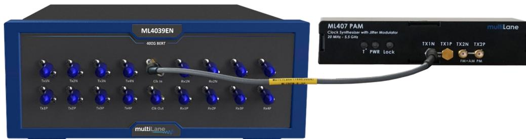
Figure 12: JTOL Test Setup
