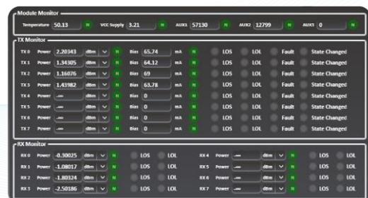
Figure 1: Digital Diagnostic Monitoring (DDM) tab
