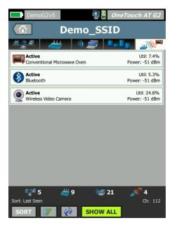
Figure 25: Unique Interferer analysis classifies sources of non-802.11.
