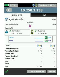
Figure 22: IP address of Test Accessories can be manually entered or download from Link-Live for easy selection.
