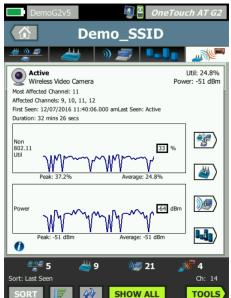
Figure 26: Detailed information about a specific interference source.
