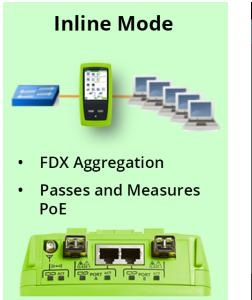
Figure 29: Inline packet capture simplifies documentation of client application problems without TAPs or SPAN ports.
