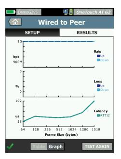
Figure 12: End-to-end path performance measurement validates link readiness and SLA compliance.
