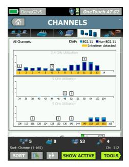
Figure 23: Analyze Wi-Fi health by each available channel.
