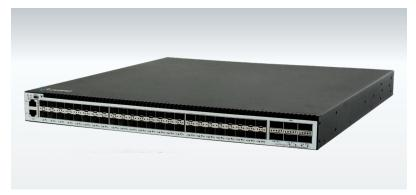
The Packetmaster EX484-3 is a high performance network packet broker that aggregates, filters, duplicates, load balances network traffic to security, monitoring and management tools based on 4500 possible rules. The Packetmaster EX484-3 supports OSI Layer 2, Layer 3 and Layer 4 header modifications including stripping, adding, and modifying VLAN tags, MPLS labels, MAC addresses, IP addresses and Port numbers.
