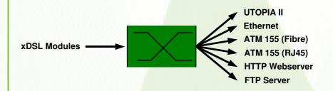
The internal data processing allows configuration of VPI/VCI interfaces, protocol selection, IP, Gateway, Net mask. 1Mbyte of internal memory has been allocated to uploadable website data. An applet within the pre-loaded website provides HTTP and FTP upload and download capability. The website allows muliple simultaneous accesses over the xDSL connections.
