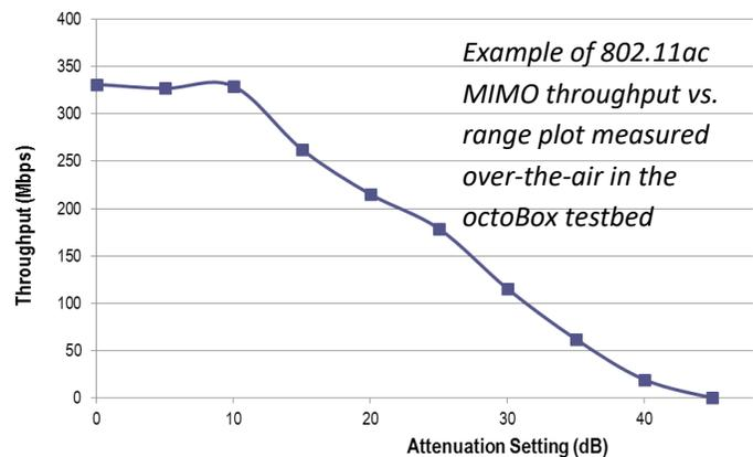
*Example of 802.11ac MIMO throughput vs. range plot measured over-the-air in the octoBox testbed*
