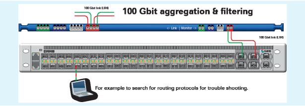
The Packetmaster EX32100 supports 8000 filters that can classify traffic. These filters can be used to redirect a selected part of the traffic to a low bandwidth monitoring tool, like a PC with Wireshark to trouble shoot an issue on a 100 Gbit link (such as a routing problem).
