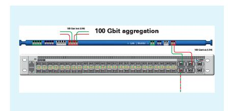
The EX32100 receives traffic from a 100G live link via the monitor ports of an inline TAP.
