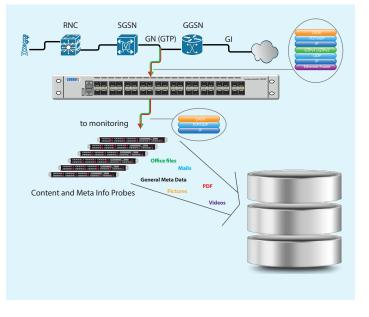
connect simple monitoring devices (Laptop & Wireshark) to analyse the traffic. The Sessionmaster forwards traffic in a small portion and therefore user can capture it with a small capturing device.
