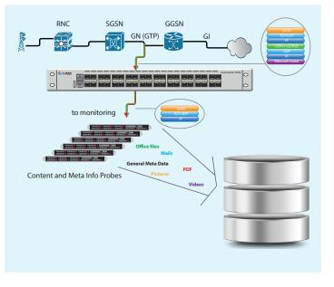
you can connect simple monitoring devices (Laptop & Wireshark) to analyse the traffic. The Sessionmaster forwards traffic in a small portion, and therefore the user can capture it with a small capturing device.
