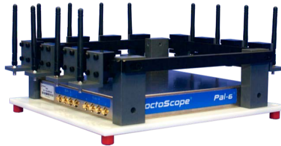
Pal-6 open with the antenna subsystem
