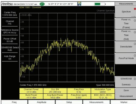
**RF Measurement – Occupied Bandwidth**
