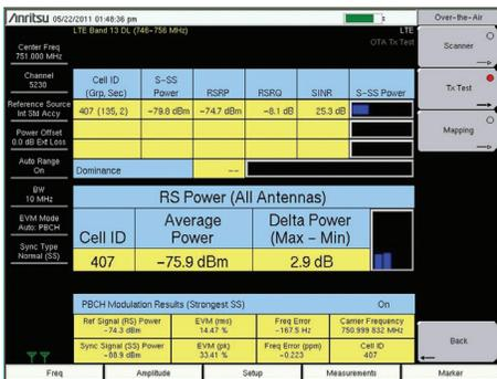
**Over-the-Air Measurements – Tx Test**
