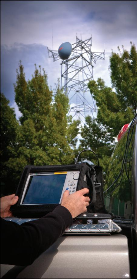
LMR Master testing from a service vehicle
