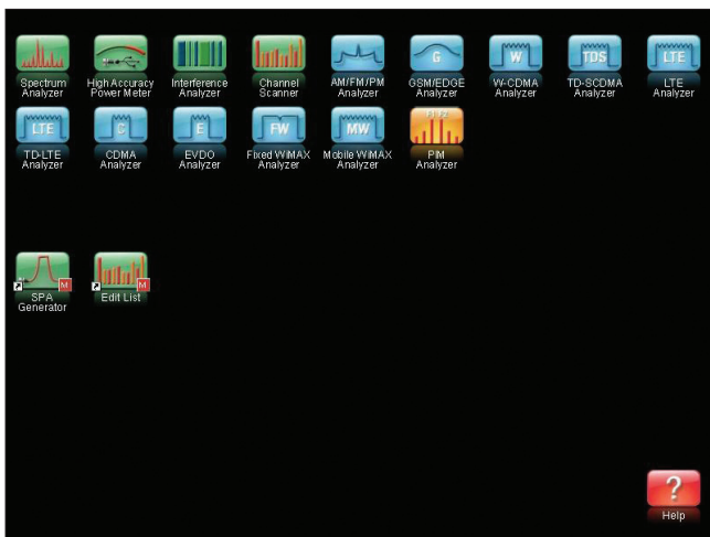
The MS2720T has a touch menu with user-defined shortcuts
