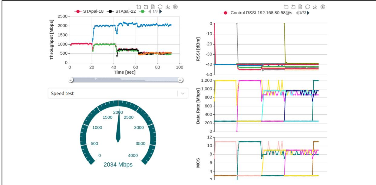
Adding a third STA increases the aggregate to 2300 Mbps. Here the gain is not quite so dramatic, but each of the three STAs is still receiving 760 Mbps. Addition of a fourth STA results in a slight decrease of the aggregate throughput to 2100 Mbps – nevertheless each STA is receiving 525 Mbps, a two-fold increase over SU operation.
