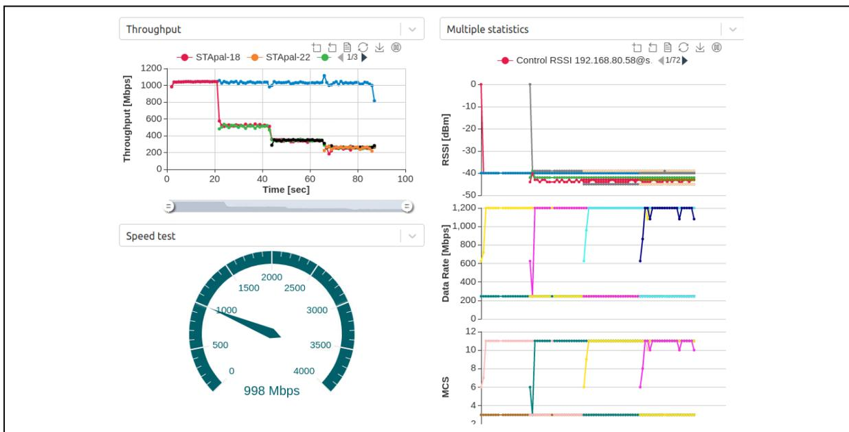
We repeat the experiment, this time with MU-MIMO switched on.
