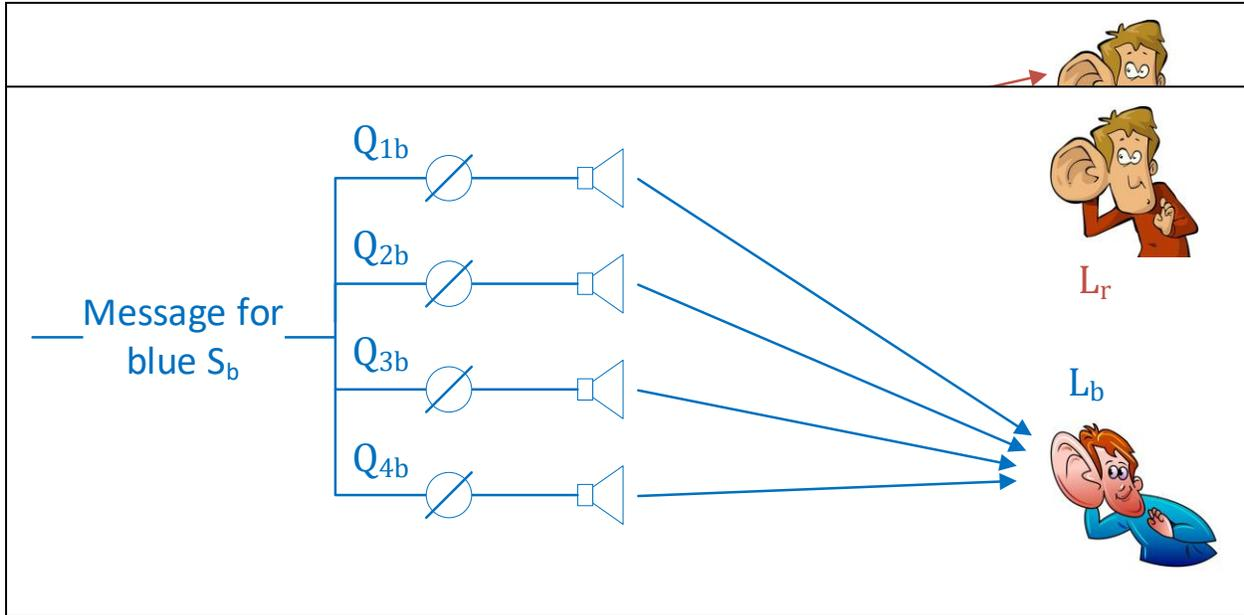
Similarly we select a set of phasors  $Q_{1b}$  through  $Q_{4r}$  to maximize the signal for listener  $L_b$  while minimizing it for listener  $L_r$ .
