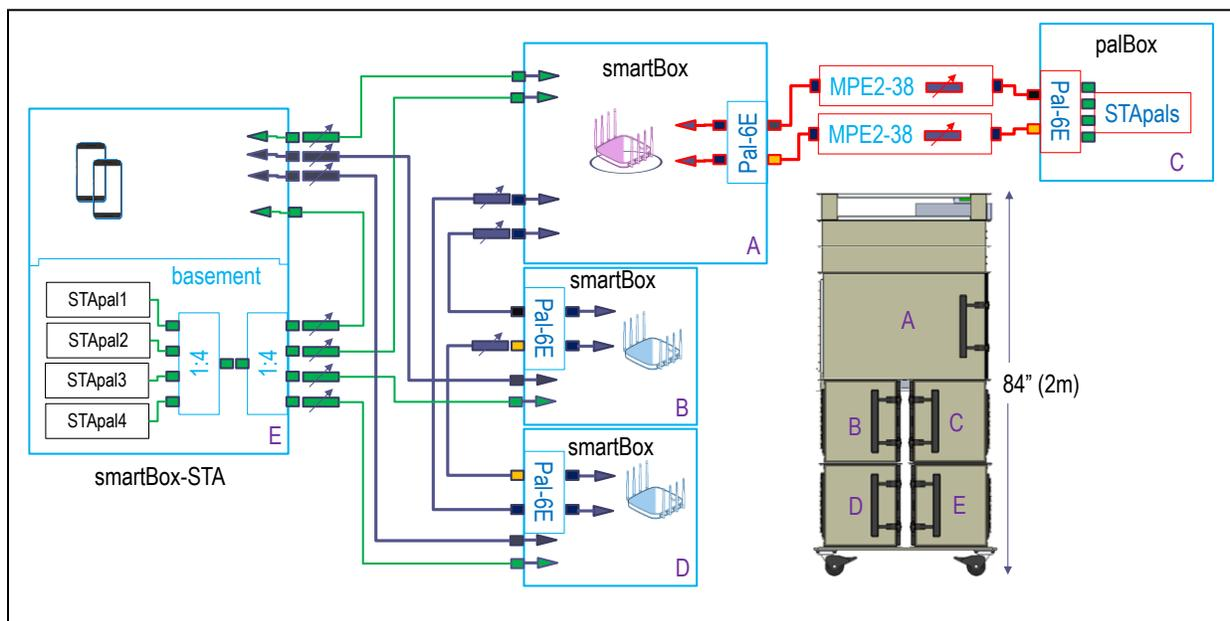
The STApal is a fully contained STA based upon the Intel AX210 chipset, running either Windows or Linux on its own hardware platform, and is able to be used as a STA or a sniffer probe. The palBox contains 16 self-contained STApals which makes it useful for OFDMA and MU-MIMO testing.
