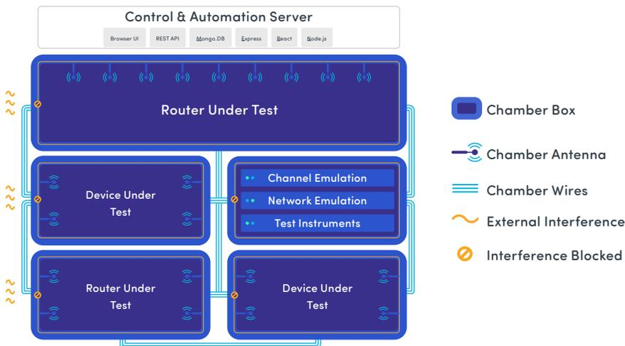
The Octobox Stack provides a modular approach to testing that includes automated testbeds with isolation chambers, antennas, emulators, and test instruments that can be rapidly configured and deployed.
