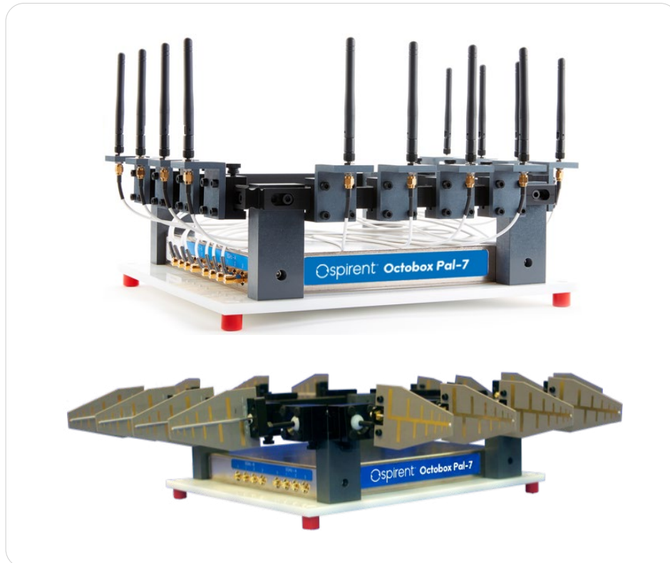
Open antenna system can be configured with any of the Octobox antennas
