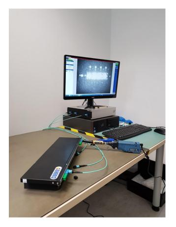
Cubro has developed a proprietary measurement device (1), that can measure up to 4 fiber pairs simultaneously, using all bandwidth speeds and all wavelength frequencies. This measurement method is not only very fast but produces repeatable results on each link; this is not often the case with standard optical power meters. The reason for this is that optical power meters are normally designed to measure longer optical fibers and not those of a very short distance.
