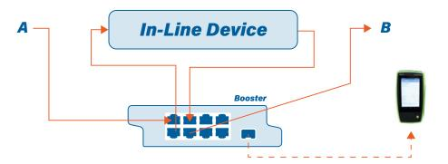
The packets going into and out of the device are aggregated and sent to the EtherScope<sup>™</sup> nXG. This provides a way to accurately measure the latency of the device between the two TAPs. Once the latency is measured, it is possible to determine if the device is the cause of the bottleneck.
