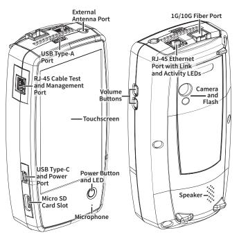
The EtherScope™ nXG is a rugged, hand-held tool for testing and analyzing copper, fiber, and Wi-Fi networks. This Portable Network Expert features applications developed by NetAlly for network discovery, measurement, and validation.
