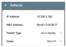
IP Address: When you enter the Reflector screen, the LR G2 automatically obtains and displays its IP address in the top field. Use this IP address to connect to the LR G2 from your main performance testing device.
