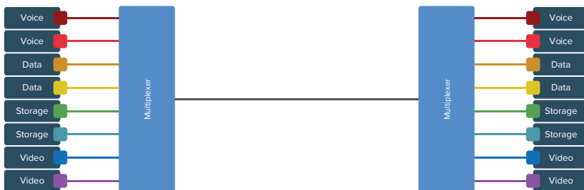
WDM allows multiple traffic signals to be transported over the same fiber
