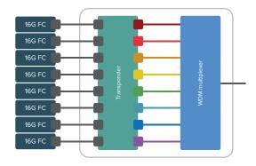
An active DWDM transponder based system provides a clear demarcation point between the data and the optical layers
