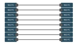
An individual fiber pair and two transceivers needed per channel
