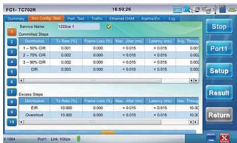
Y.1564 Service Measurement Interface
