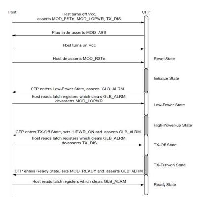
MOD\_RSTs assertion drives the CFP2 module to a reset state, at this stage the MDIO interface will be held in a high impedance state, the Host will read 'FFFF'h from any address, while host write operations will have no effect.
