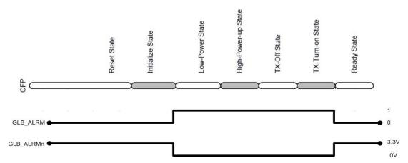
GLB \_ALRM is de-asserted during Reset and Initialize state, it is asserted in Low-Power, High-Power-up, TX-Off and TX-Turn-on states, then de-asserted again when Ready state is reached. GLB ALRMn is the hardware pin, and is the inverse of GLB ALRM.
