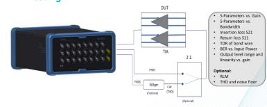
Figure 5: TIA Testing Using ML4035
