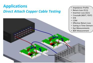
Figure 4: DAC Testing Using ML4035
