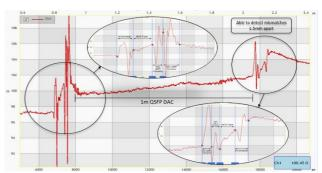
Figure 1: TDR Measurement on DAC + MCB
