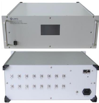
Figure 3: An RF Switch Matrix can be used to connect RF cables once.
