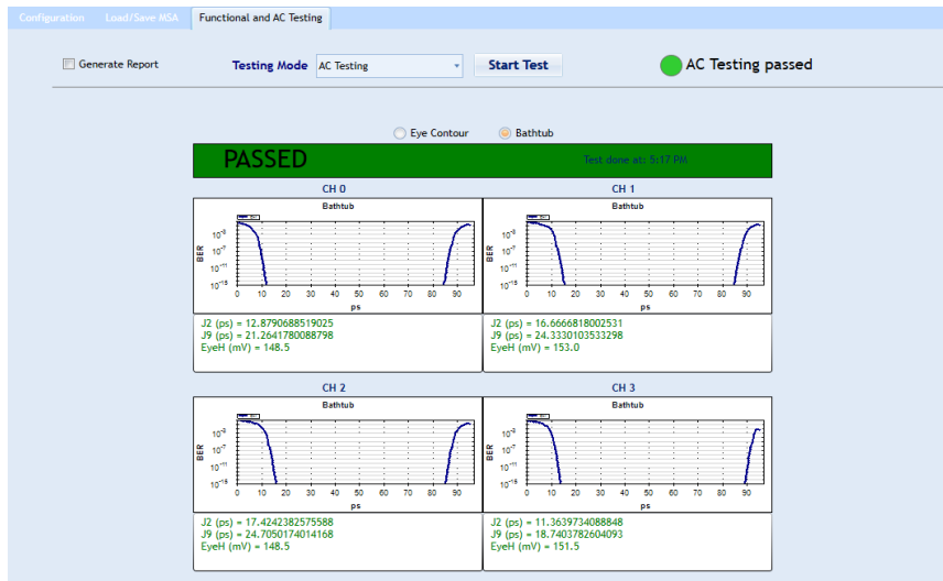
Figure 3: QSFP bathtub curves
