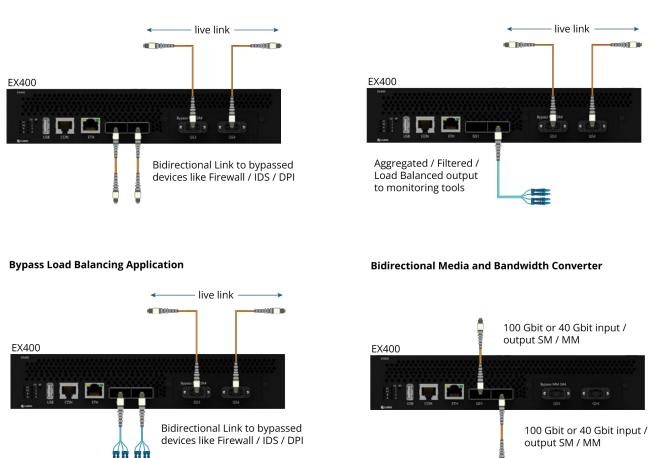
100 Gbit Bypass application for bypassing an inline firewall in case of any failure.
