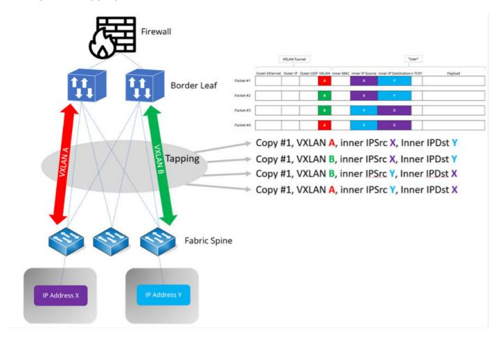
Traffic between IP X and IP Y passes the tapping two times and thus the same packets are visible twice at the tapping output. From user perspective every packet is received twice.
