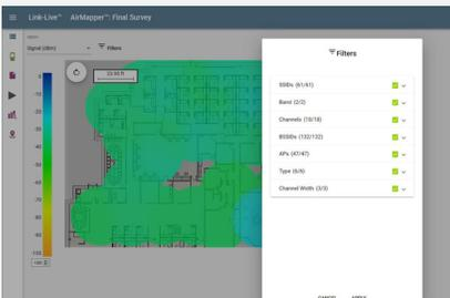
Multiple filters can be used to customize the visualization
