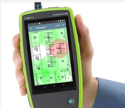
Signal propagation determines how far AirMapper will assume a given reading is applicable
