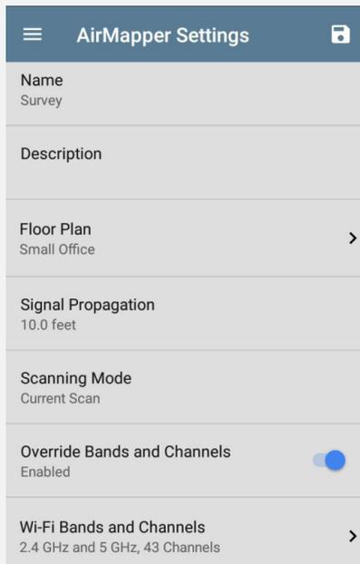
EtherScope general settings allows the user to specify a subset of channels or bands to be scanned for all applications such as Wi-Fi and Discovery. If desired the user can now select different channels and bands to be scanned as a part of the current survey independent of the general settings.
