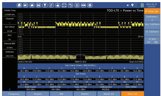
Figure 5: TDD-LTE power vs. time measurement.
