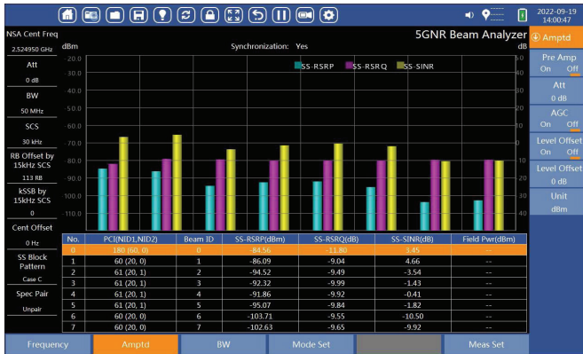
Figure 7: 5G NR FR1 beam analyzer measures up to 8 beams at once.
